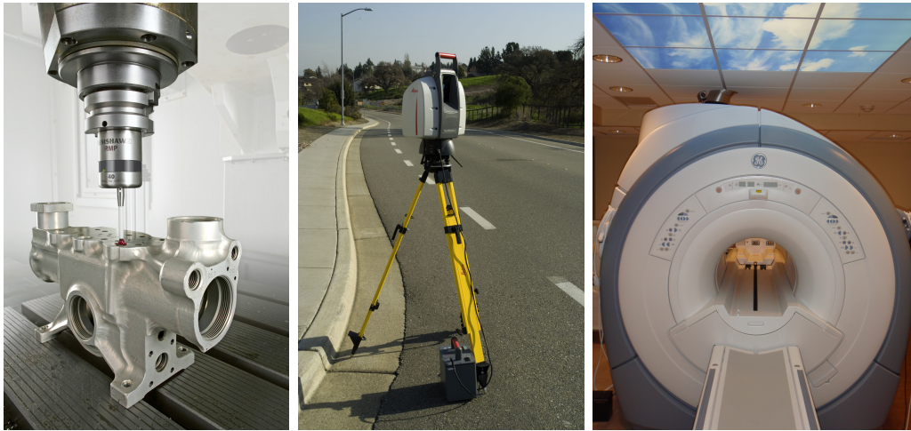
Figure 2.6: A variety of scanning technologies. (left) Touch probe. (center) Time of flight laser scanner. (right) Magnetic resonance imaging machine.
