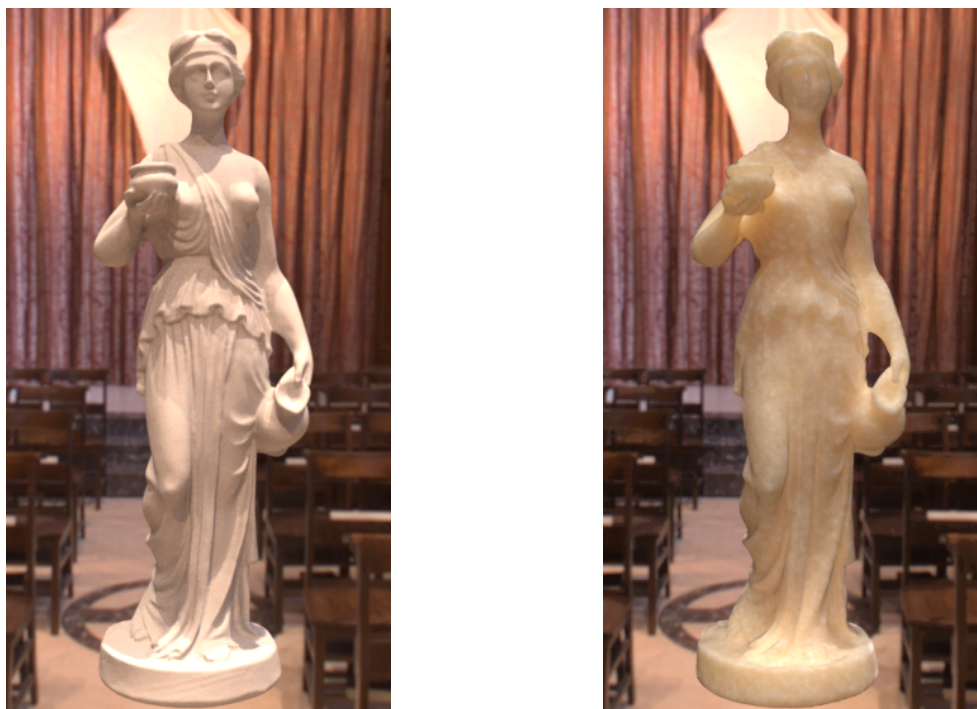
Figure 2.3: Example of an object rendered with an opaque BRDF (left), and a translucent BSSRDF (right).
