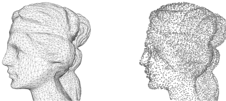
Figure 2.2: The 2D surface of a small statue represented with a connected triangle mesh and with point samples.
